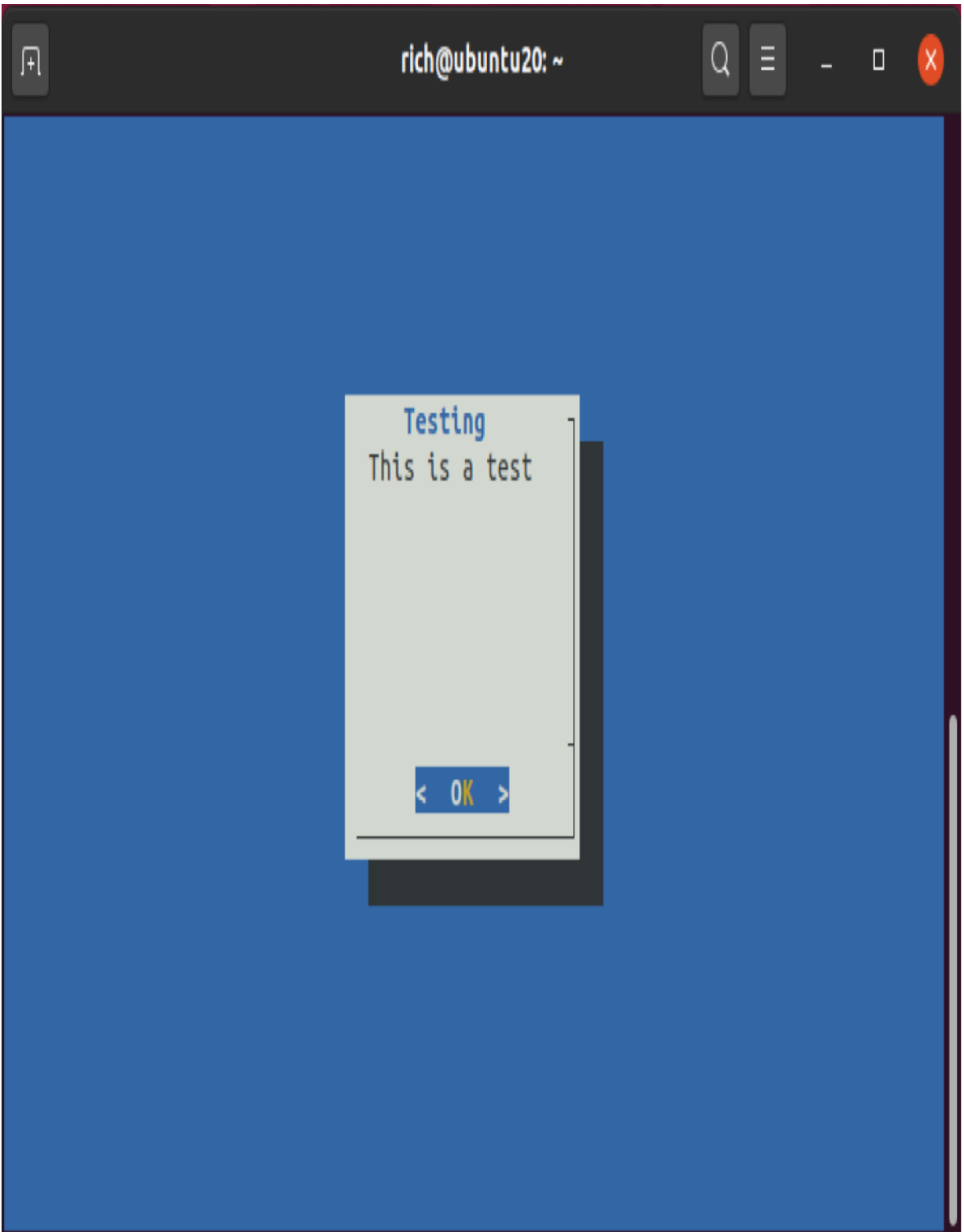
FIGURE 18-2 Using the msgbox widget in the dialog command
