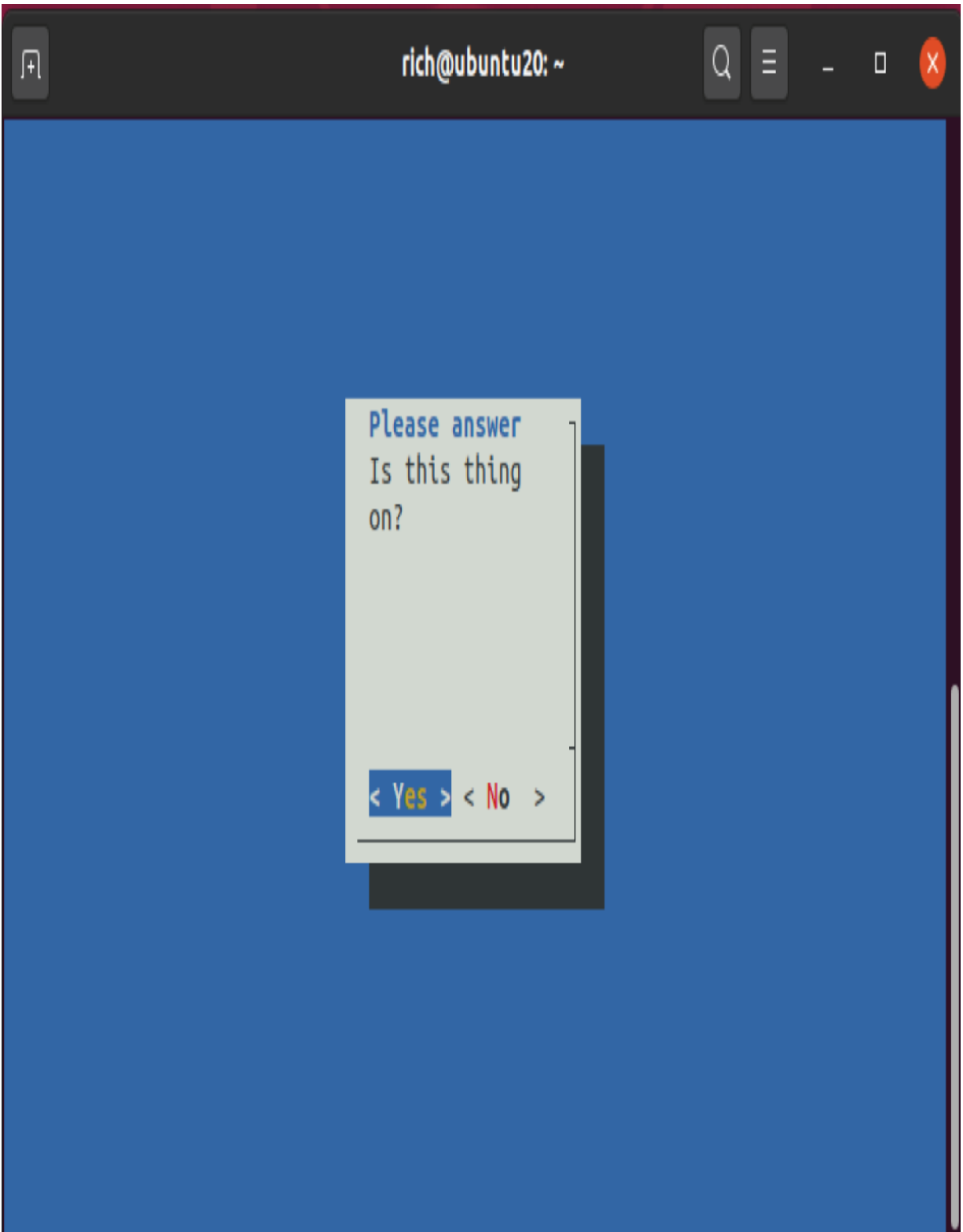
FIGURE 18-3 Using the yesno widget in the dialog command
