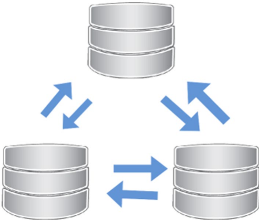
Figure 5-3. Multimaster replication topology
